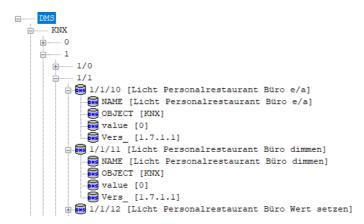
where the root (in the example: KNX) can be adapted. For visualization and operation the DMS addresses (Ex: "KNX:1:1/1:1/1/12:Switch" can be used.
