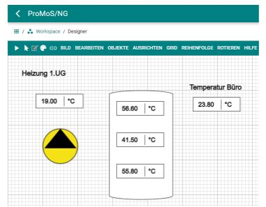
All temperatures and the pump are already animated. Images can be saved and loaded. The start image can be defined. The image format is new JSON and can be edited by hand like the old format (surely not recommended - search and replace in text files works as before).
